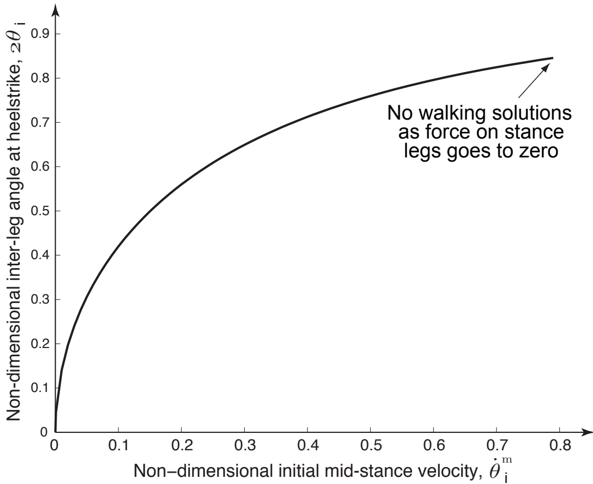
Figure 6: One step capture point The external disturbance is modeled as a non-zero mid-stance velocity (x-axis). The plot shows the step length (y-axis) needed for the robot to come to a complete stop (zero mid-stance velocity of the stance leg) at the next mid-stance. For high enough velocities there are no solutions because the reaction force on the stance leg goes to zero. If we allow for a flight phase, the solution is unbounded.
