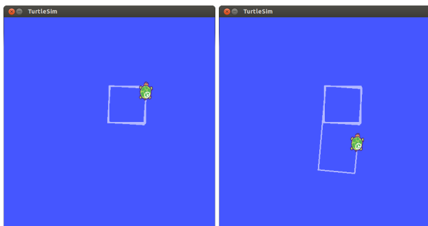
Figure 9.3: [left] A turtlesim turtle responding to movement commands from draw_square. Those movement commands are also recorded by rosbag. [right] By replaying the bag, we can send the same sequence of messages to the turtle.
