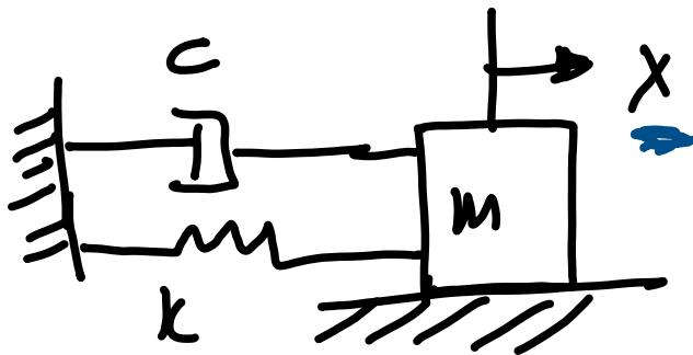
Equation of motion  $\ddot{m}x + c\dot{x} + kx = 0$
