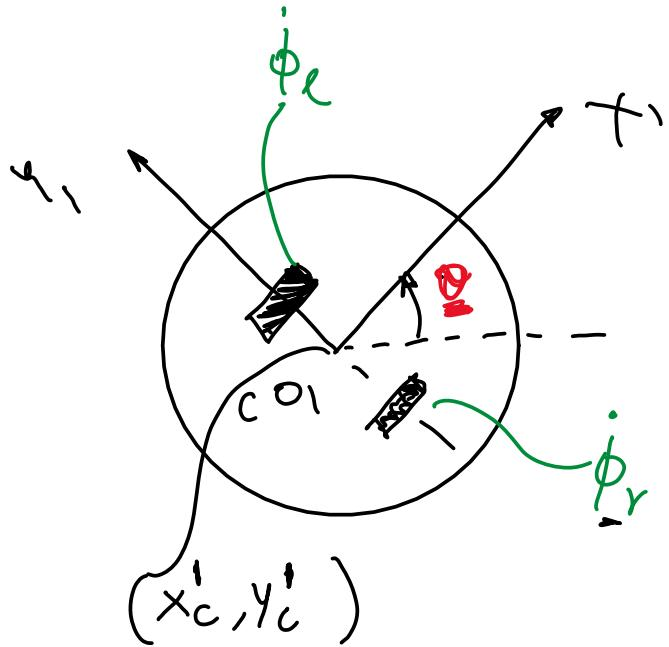
Part 2: Effect of rotation due to different speeds
