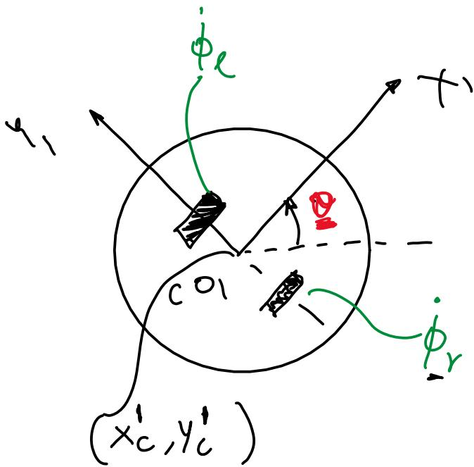
$$\begin{aligned} \phi &= \text{constant} \\ s &= r\phi \\ \dot{s} &= r\dot{\phi} \end{aligned}$$
