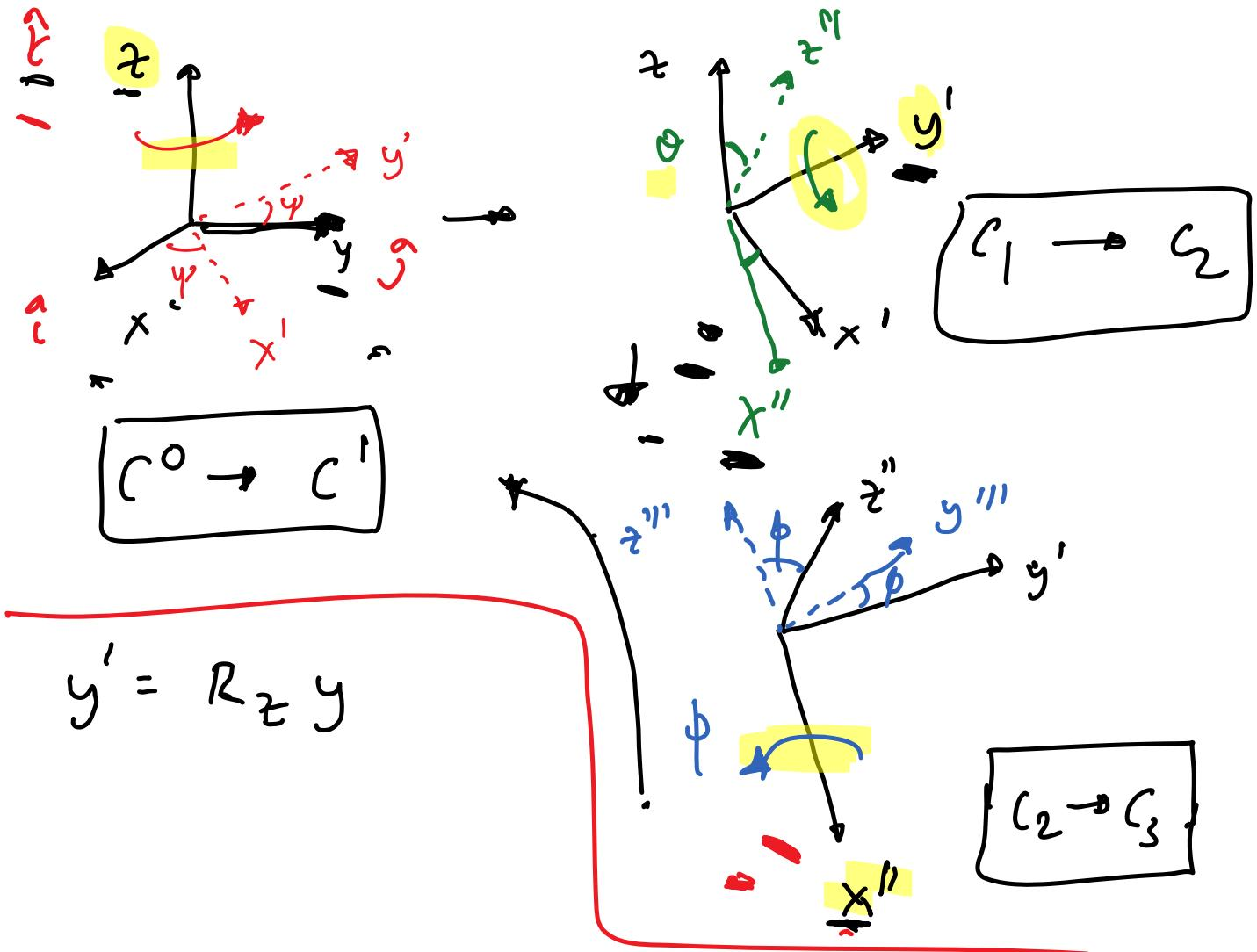
$$\begin{aligned}\vec{\omega} &= \dot{\psi} \hat{z} + \dot{\theta} \hat{y}' + \dot{\phi} \hat{x}'' \\ &= \dot{\psi} \hat{k} + \dot{\theta} (R_z \hat{j}) + \dot{\phi} (R_x R_y \hat{i})\end{aligned}$$
