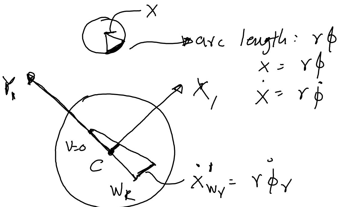
$$\left\{ \begin{array}{l} \dot{\phi}_L = 0 \\ \dot{\phi}_R \neq 0 \end{array} \right. \rightarrow \dot{x}'_C = 0.5r\dot{\phi}_y$$
