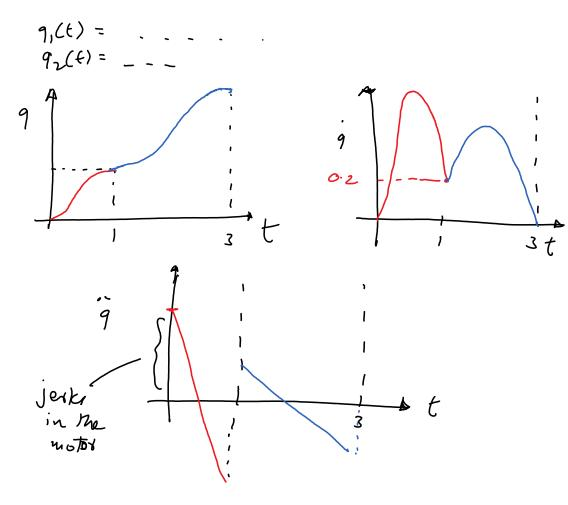
Example 2: Find a time based parameterization for a revolute joint of a manipulator. The joint should move from 0 to 0.5 rad from time t= 0 to t=1 sec followed by movement from 0.5 rad to 1 rad in from t=1 to t=3 secs. Also, the velocity of the joint at the start of motion (t=0) and end of motion (t=3) should be 0 and the acceleration of the joint at the intermediate point (t=1) should be continuous. Assume two minimal order polynomials of time, one for each movement.
