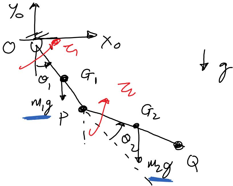
Find the torques  $\tau_1$  and  $\tau_2$  such that the double pendulum is in static equilibrium
