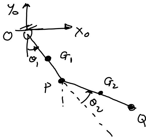
$$\begin{aligned} q &= \begin{bmatrix} \theta_1 \\ \theta_2 \end{bmatrix} \\ \dot{q} &= \begin{bmatrix} \omega_1 \\ \omega_2 \end{bmatrix} \end{aligned}$$
