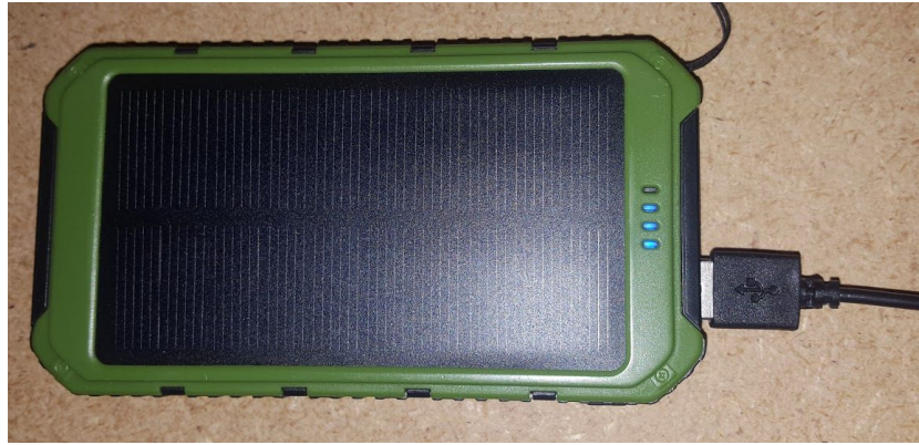
Figure 6: 10,000 mAh Portable Battery Pack with USB lamp connection
