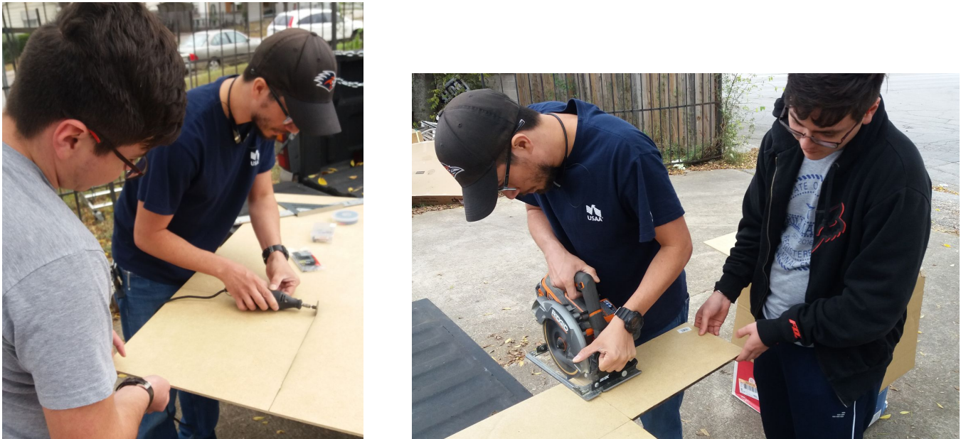
Figure 2: Cutting MDF box housing with a Dremel (Left) Cutting using a circular saw (Right)
