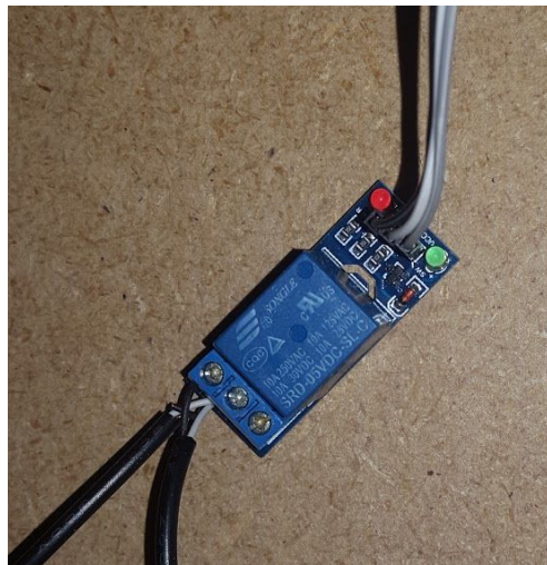
Figure 5: Relay with all wire connections
