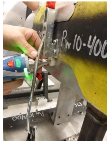
Figure 1. Sheet Metal Part Traced by Faro
