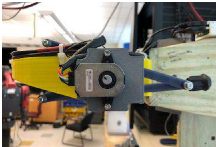
Figure 4.2. Correct shaft position of the outer motor after calibration.
