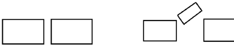
Figure 35. Assuming the rectangles are robots, the figure above shows that the three robot design can fail if the space between the two robots that the robot behind is trying to leapfrog over has too much distance between one another.
