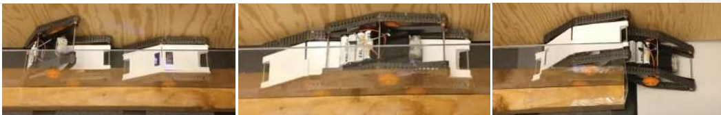
Figure 6. Three robot design with a motor disabled robot included
