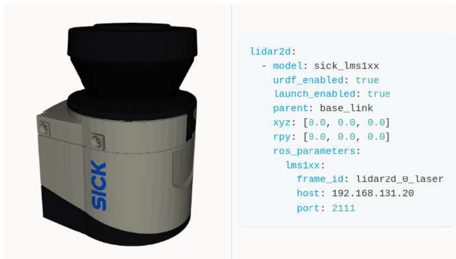
Figure 9: SICK LMS111 2D LiDAR sensor
