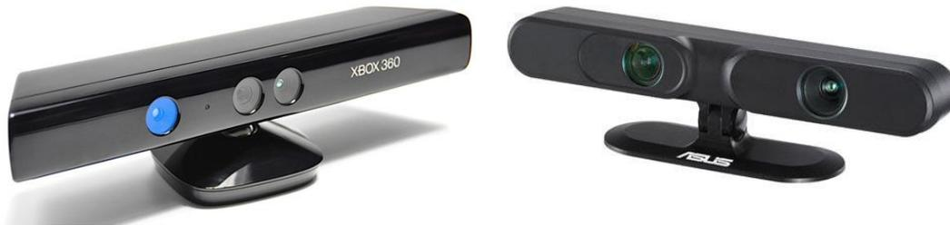
Figure 1: Microsoft Kinect and ASUS Xtion RGB-D cameras
