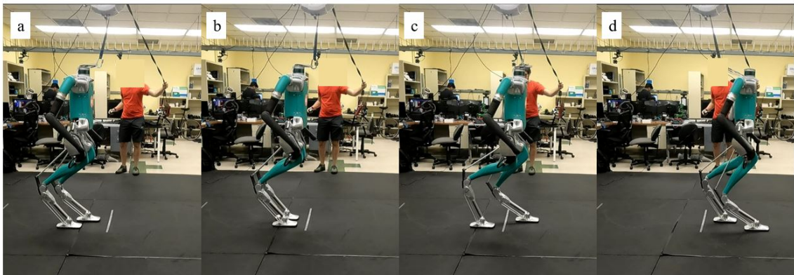
Figure 71: Asymmetric stepping hardware experiment. (a) the robot takes a nominal step size followed by (b) a short asymmetric step to drive the COM forward, then (c) a long step is taken to slow down the velocity of the COM and step over the obstacle on the floor and finally (d) the robot successfully clears the obstacle.
