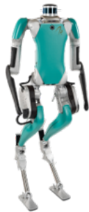
Figure 31: Robot model: Digit bipedal robot with 30 degrees of freedom and 20 actuated joints.
