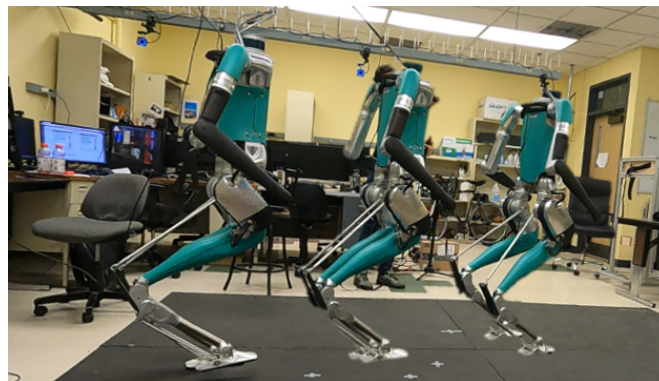
Figure 56: v_{des}^+ tracking hardware experiment using the NH-LIPM controller.
