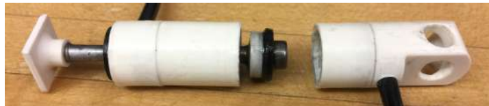
Figure 34: Longitudinal Stress Failure of a Dynamically Tested Actuator Prototype
