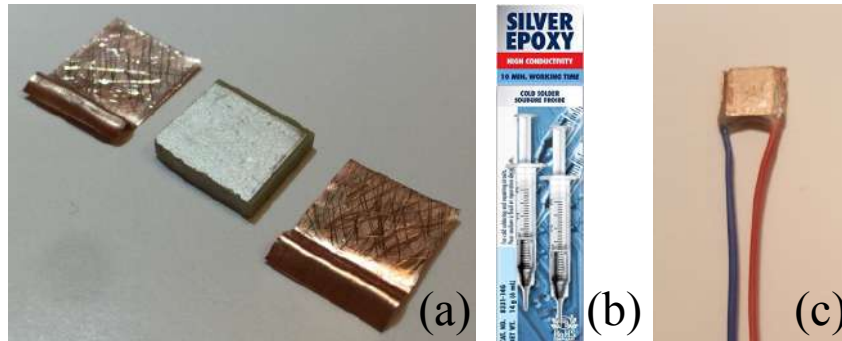
Figure 26: Images of the Piezoelectric Crystal (Center) with Two Copper Electrode Sheets, Silver Epoxy, and Composite Sensor Structure
