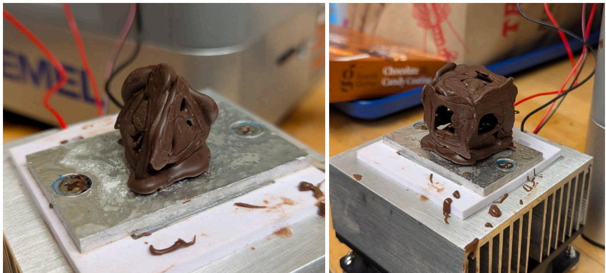
Early successful multi-layer prints, a solid shape and a hollow cube, achieved by pausing between layers to allow cooling (~30 sec–1 min), manually flipping, and continuing the print, marking a breakthrough in the layering process ( Apr. 2025 )
