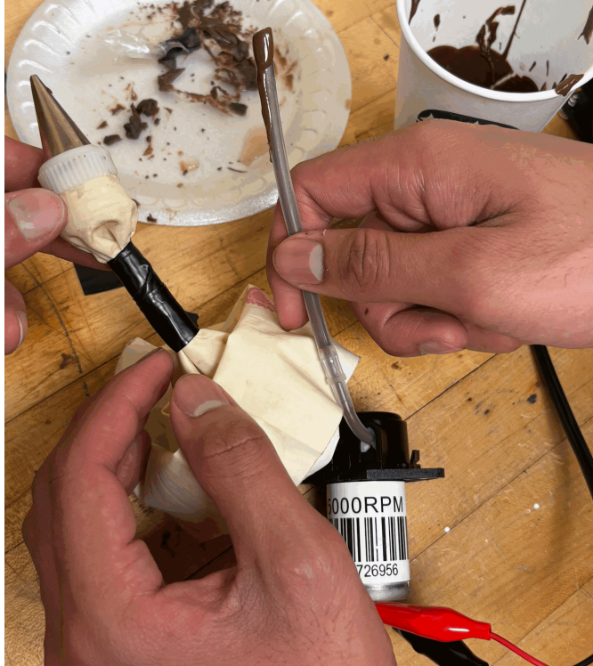
Team members holding an early iteration of the nozzle system to push chocolate through the white housing. Later versions improved materials, tighter seals, and heating ( Mar. 2025 )
