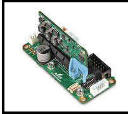
Figure 19: EPOS2 Motherboard & 36/2 Module [5]
