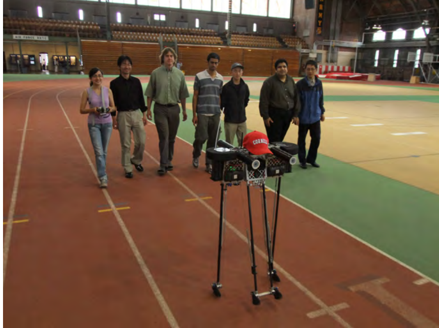
Figure 3: Ranger’s ultra-marathon walk. On 1-2 May 2011 [43], Ranger walked non-stop for 40.5 miles (65 km) on Cornell’s Barton Hall track without recharging or being touched by a human. Some of the crew that worked on Ranger are shown walking behind Ranger during the 65 km walk. The walk lasted for 30 hr 49 min. The robot speed was 1.32mph or 2.12kmph. Total energy usage was 16W of which 11.3 W was used by motors and the rest 4.7 W was used by the computers and sensors. The TCOT was 0.28. This was further reduced to 0.19 after we did energy optimization to compute the nominal trajectory.
