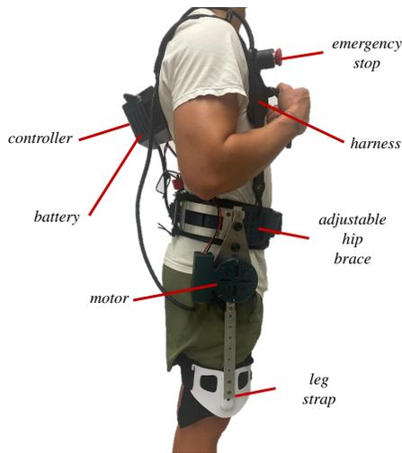
**FIGURE 2.** A DETAILED IMAGE OF THE HIP EXOSKELETON HIGHLIGHTING ITS PRINCIPAL FEATURES, INCLUDING THE 24V BLDC MOTOR FOR VARIABLE STIFFNESS CONTROL, ADJUSTABLE STRAPS FOR A SECURE FIT, AND RIGID PLASTIC BRACES. THE DESIGN IS OPTIMIZED TO SUPPORT HIP FLEXION AND EXTENSION DURING SQUATTING MOVEMENTS.
