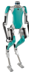
Fig. 1: Robot model: Digit bipedal robot with 30 degrees of freedom and 20 actuated joints.
