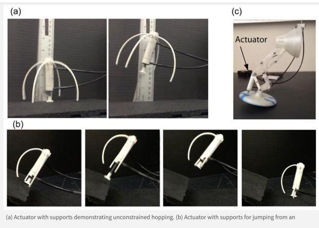
inclined surface to the ground. (c) Actuator incorporated into legged robot based on Disney/Pixar Luxo lamp character.
