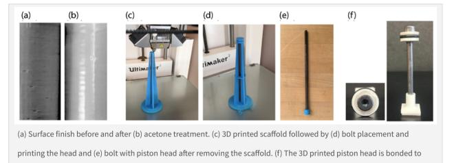
piston rod by an adhesive. The O-ring is manually placed in the groove on the piston head.
