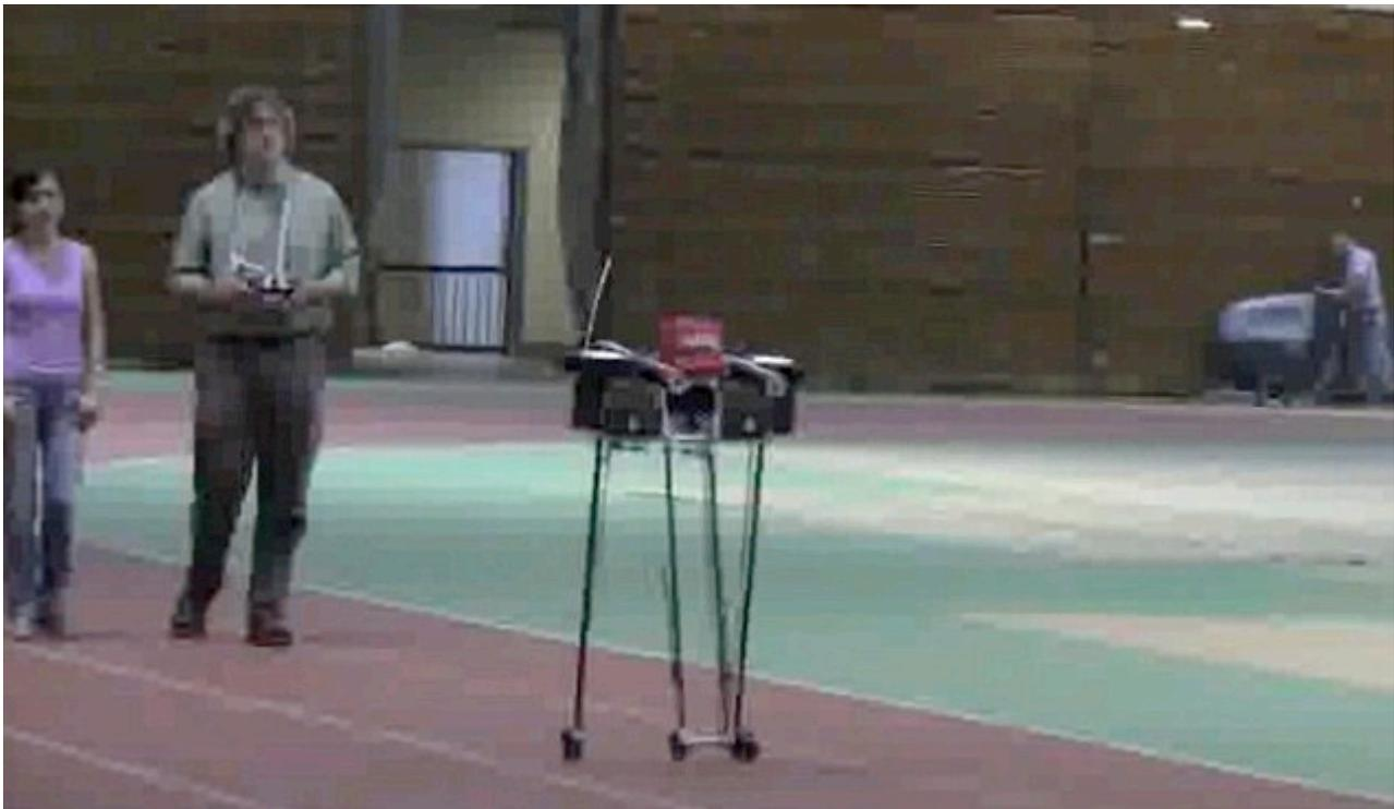
**Marathon: Cornell University's Ranger robot broke the world record for continuously walking without needing to be recharged or even touched by engineers**
