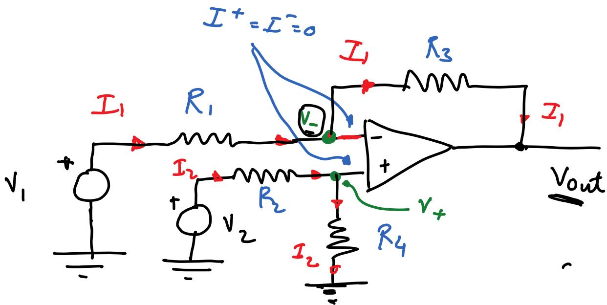
$$V_- = V_+ \quad (\text{op-amp assumption})$$
