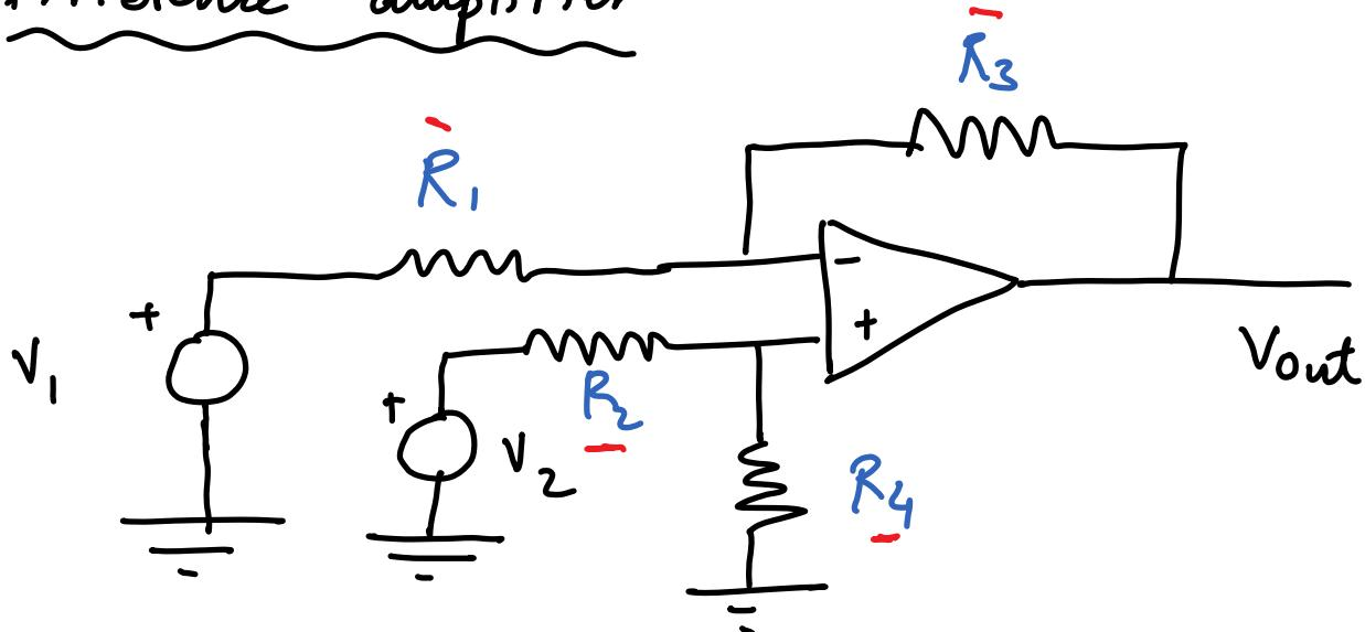
Compute  $V_{out} = f(V_1, V_2)$  and resistors
