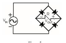
Build the circuit shown above in TinkerCAD. Use  $R = 100k\Omega$ . Using the function generator to apply a sinusoidal wave of 10 V peak-to-peak at 100 Hz. Set up the oscilloscope to measure and plot  $V_{\rm in}$  and  $V_{\rm out}$  as function of time. Show the circuit and the plot to the teaching assistant.
