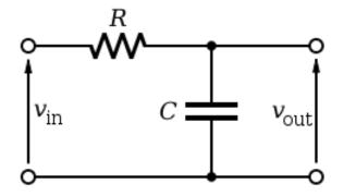
The theoretical cut-off frequency (in hertz) for a low-pass RC filter in terms of R and C is given by  $f_c$  given by
