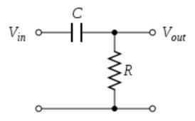
The theoretical cut-off frequency for a high-pass RC filter in terms of R and C is given by  $f_c$  given by
