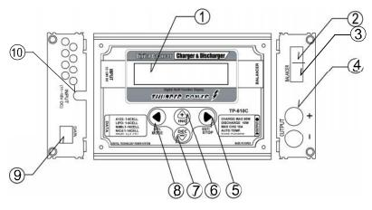
1: LCD screen 2: Upgrade connector 3: BL-2 (balance tap) connector 4: Charge Output 5: Enter/Stop button 6: INC button 7: DEC button 8: SEL/MODE button 9: Data port 10: Power input
