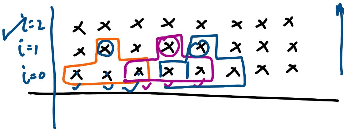
$$\alpha \left[ \frac{T_{i,j+1} - 2T_{i,j} + T_{i,j-1}}{\Delta x^2} \right] = \left[ \frac{T_{i+1,j} - T_{i,j}}{\Delta t} \right]$$
