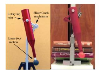
Figure 1: Modular robotic leg: Left: Machined from aluminum; Right: 3D printed. This one is half the size of the one shown on the left.
