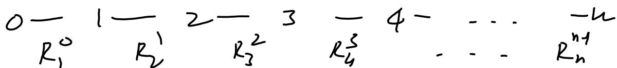
$$w_n^o = w_i^o + R_i^o w_2^1 + R_2^o w_3^2 + \dots + R_{n-1}^o w_n^{n-1}$$
