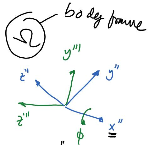
$$\begin{aligned}\omega &= \dot{\psi} \hat{z} + \dot{\theta} \hat{y}' + \dot{\phi} \hat{x}''' = R_z R_y \hat{e} \\ &= \dot{\psi} \hat{k} + \dot{\theta} R_z \hat{j} + \dot{\phi} R_z R_y \hat{u} \\ &= \dot{\psi} \hat{k} + R_z \dot{\theta} \hat{j} + R_z R_y \dot{\phi} \hat{u}\end{aligned}$$
