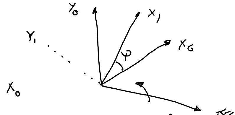
$$R_2(\psi) = R_1^0 = \begin{bmatrix} \cos \psi & -\sin \psi & 0 \\ \sin \psi & \cos \psi & 0 \\ 0 & 0 & 1 \end{bmatrix}$$
