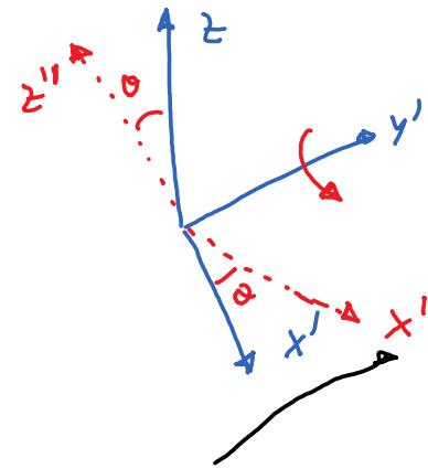
$$\boxed{\underline{C^0} = R_z(\psi) \underline{C^1}} \quad \text{world frame} \quad \text{Body frame} \quad \textcircled{I}$$
